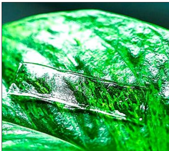
Adhesive gel sticks easily to plant surfaces and can be loaded with medicines.
